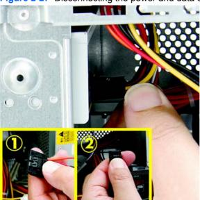
Figure 2-27 Disconnecting the power and data cables
